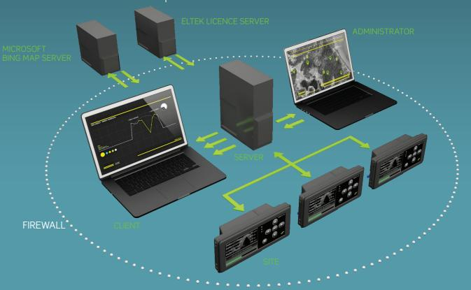
Communication between the server and the on-site controllers takes place within the boundaries of a firewalled supports all major communication
